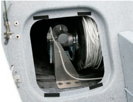
Winch unit installed in Dynamic
