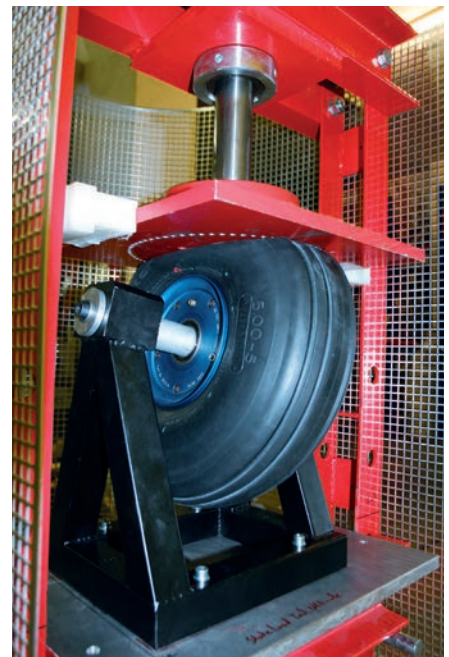
Static load test of a complete wheel
