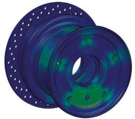
FEM-based analysis of Penta disk brake wheel
