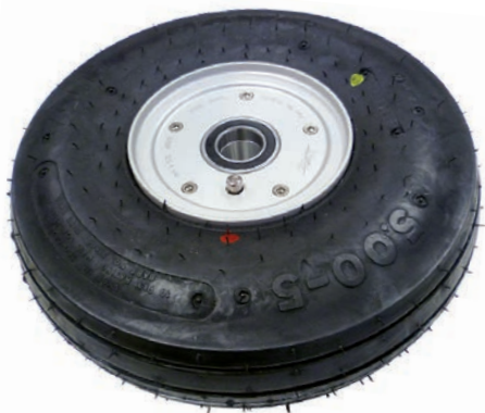
Red Dot marking on larger aircraft tires
